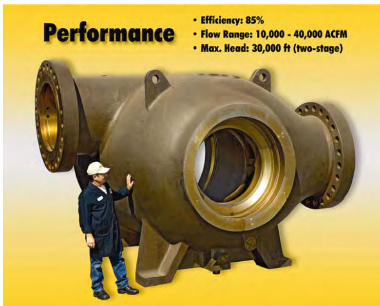
Figure 6. C85 Centrifugal Gas Compressor
