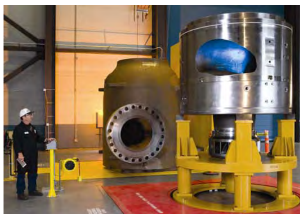
Figure 19. Gas Compressor Assembly
