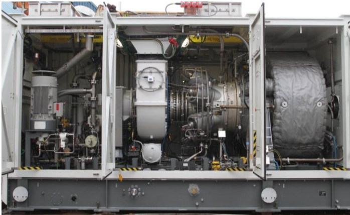
Figure 8a: SGT-400 package as being used for SGT-300 TS for improved serviceability
