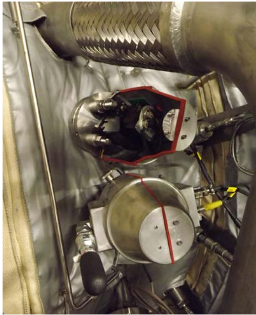
Figure 3: Infrared cameras installed on the gas turbine, two out of four visible.
