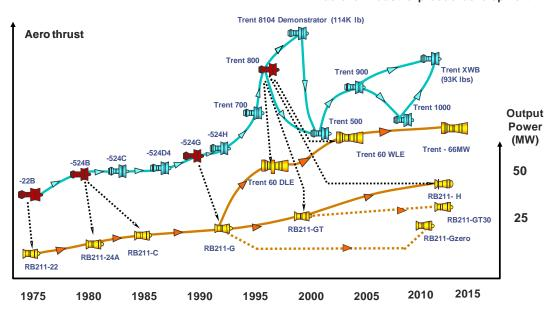
**Figure 5**. Shows the derivation of energy gas turbines from their aero power plants
