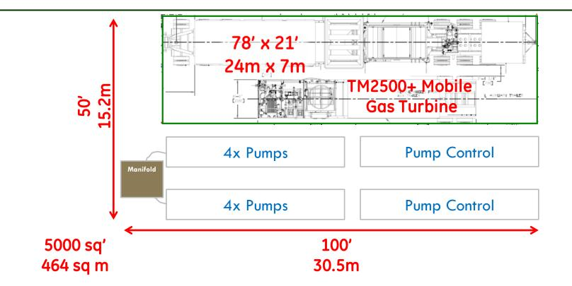
40% less area required for power train and pumps using the EWS/GE System
