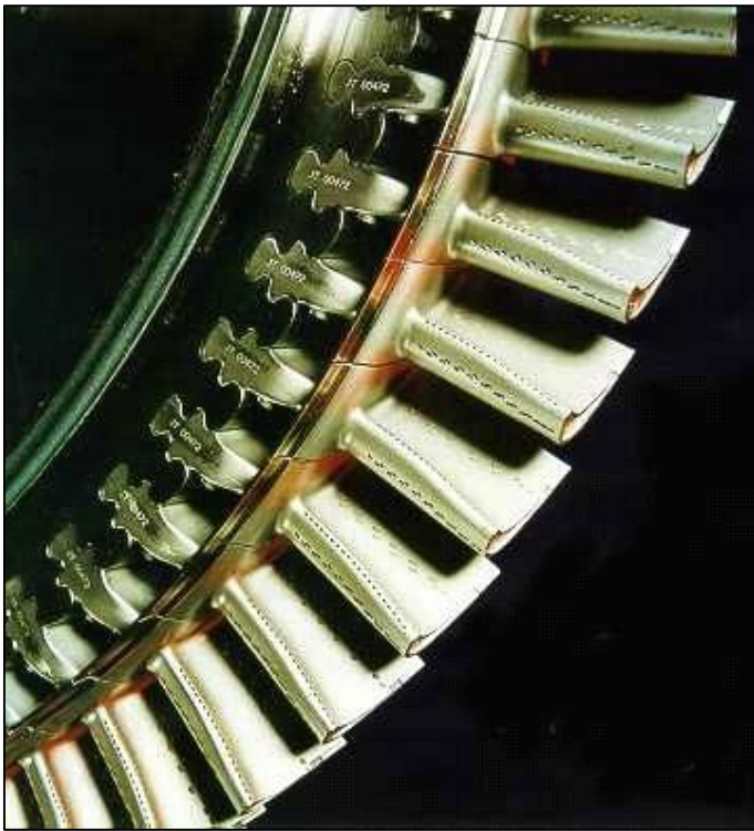
Turbine row assembly, showing blade attachments to the rotating disk, and blade cooling air exit holes
