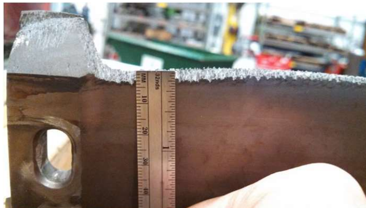
Figure 26: L-0 As found In-Service Blade
