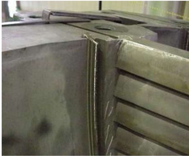
Figure 22: Tip Seal Segments Installed in Stationary
