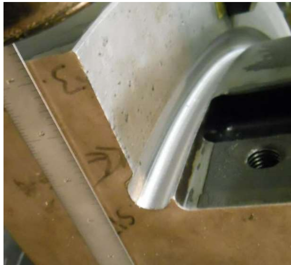
Figure 5: Machining of N2 Main Fit Radii
