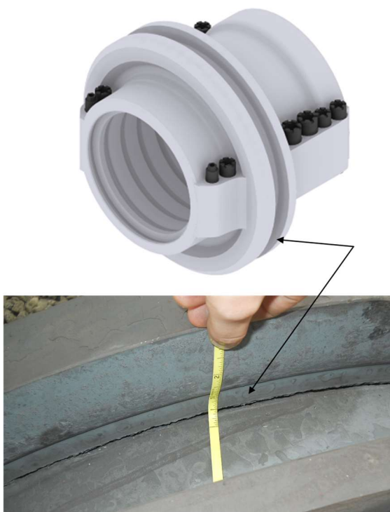
Figure 4: N2 Packing Casing Ledge Cracks
