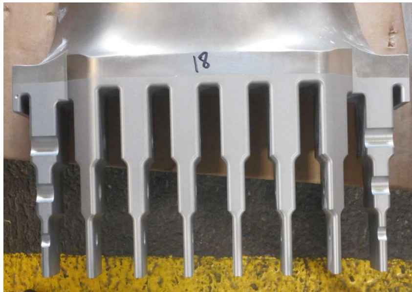
Figure 25: L-0 Pin Finger Root Modification
