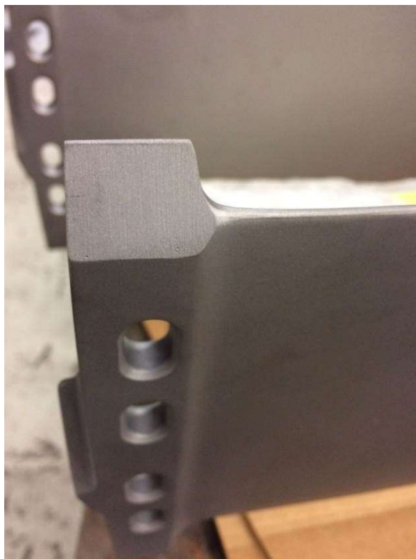
Figure 27: L-0 As Repaired In-Service Blade
