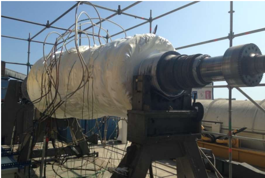
Figure 10: HP / IP Rotor Preparing for Straitening Process
