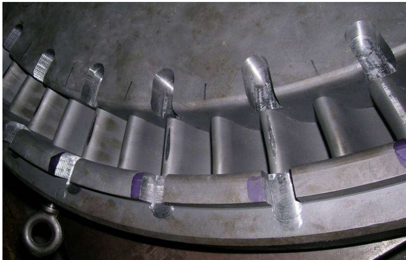
Figure 9: Preparation For Diaphragm Stiffener Welding
