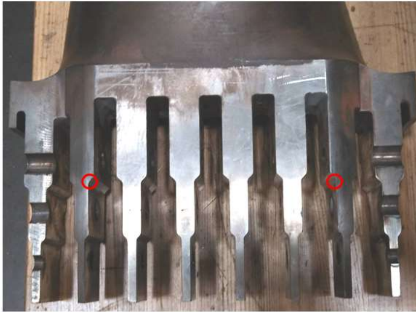
Figure 24: L-0 Pin Finger Root Cracking Locations
