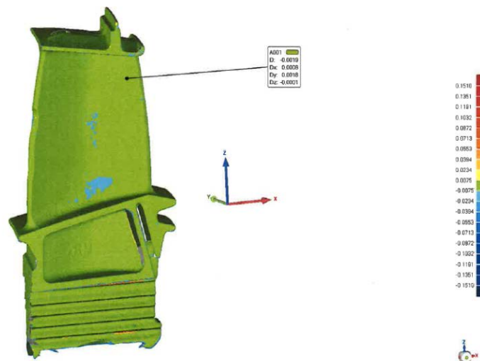
Figure 7: Typical CMM deviation analysis of a blade showing no significant dimension change/distortion after solution heat treatment. Units: inches.
