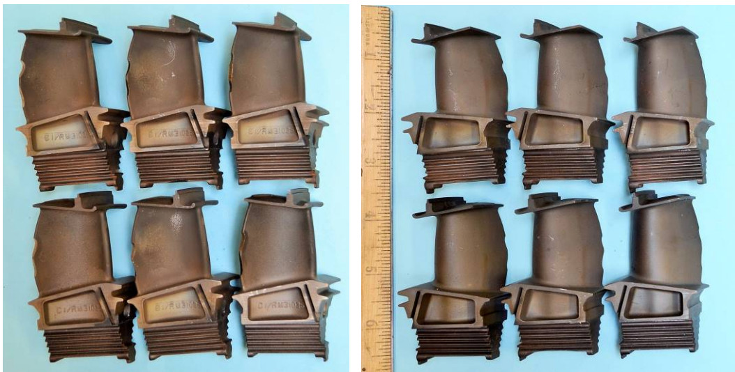
Figure 2: As received appearance of the blades used for repair demonstration (concave and convex side). Note that the blades had been 'notched' on the trailing edges identifying them as unserviceable.
