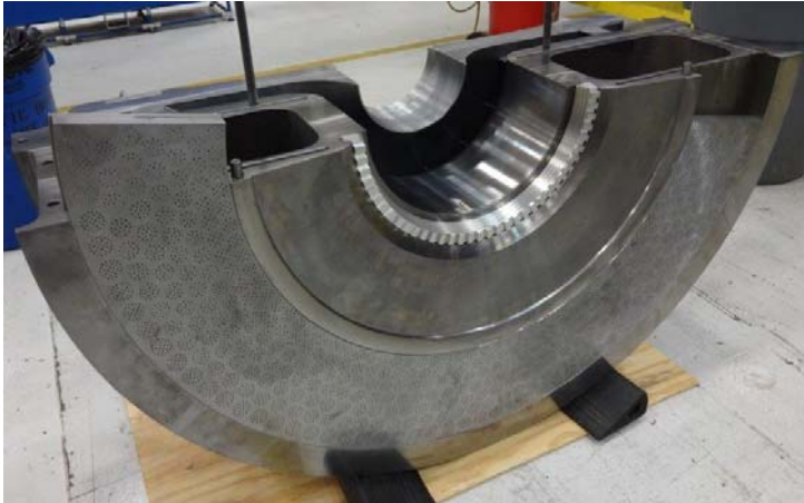
Figure 5: Photo of one half of a flat plate acoustic array.
