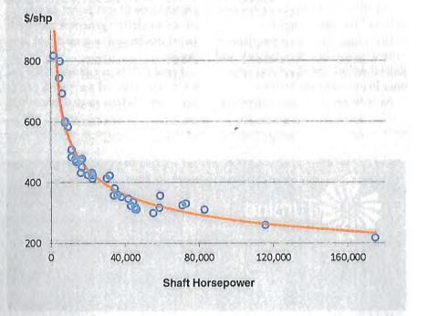
of supply includes gas turbine, reduction gearbox (when needed), inlet air filter, auxiliaries, and dry low NOx combustion, when available:
