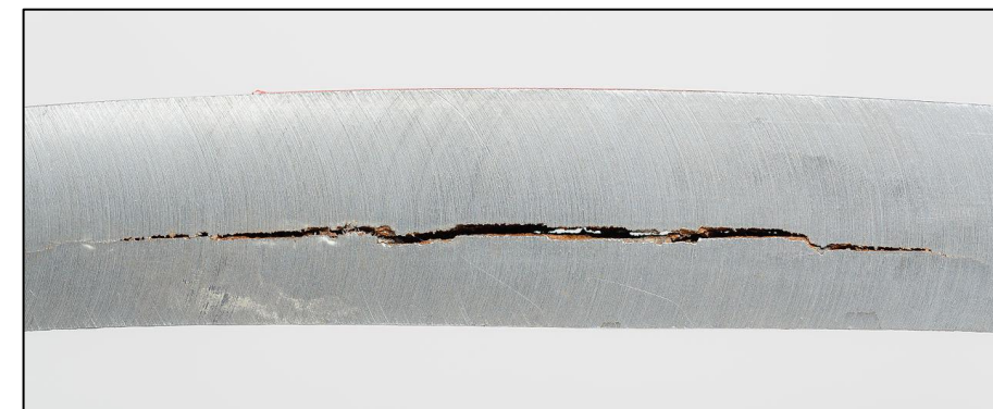
Figure 1: Hydrogen Induced Crack [Uwe Aranas, Wikimedia]
