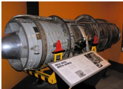
RR Olympus, from Concorde 593 Engine
